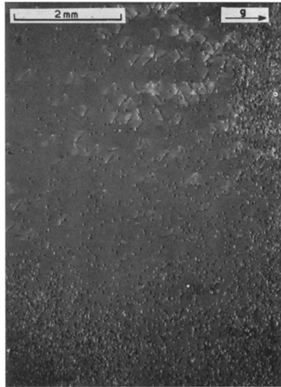
Figure 7 Symmetrical \{220\} Laue topograph of an oxidized epitaxial silicon wafer. \text{CuK}\alpha_1 radiation.
